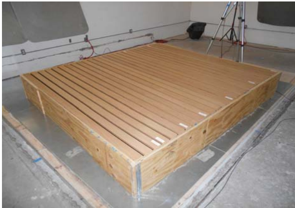
E400 test with 4" Linear Veneer (2-inch backing)
