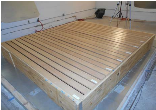
E400 test with 4-1/2" Linear Veneer (2-inch backing)
