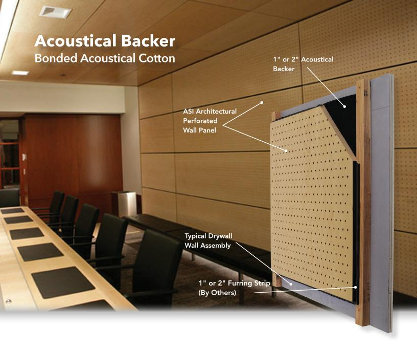
Acoustical Backer Acoustical Cotton is an economical, multipurpose, high performance, Class A fire retardant, sound absorber. It is exceptionally durable and can be used anywhere cost effective noise control or reduced reverberation time (echo) is needed. Acoustical Backer installs easily to ceilings or walls using contact or construction adhesive.
